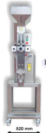
AISI 304 stainless steel frame Stainless steel jaws
